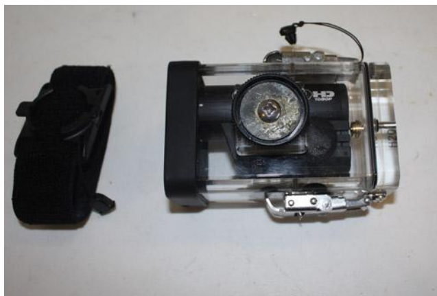
The H2OV housing with the center disk, washer, and bolt installed properly. Note the tether connected to the top clasp for the back door and on the had-strap.
