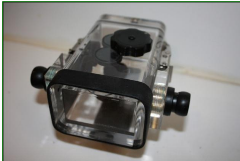
H2Ov pictures with two adhesive acrylic mounting blocks for video light arms. Placement of the block is key to assure proper operation of the latch and front guard.
